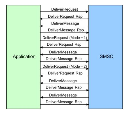
Figure 2. Flow of delivery request operations
